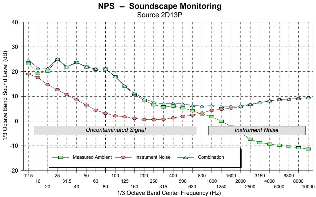
**Figure 2. 1/3-Octave Band Example of Noise Floor Contamination**
